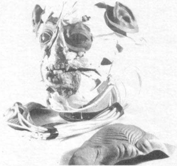
All of the control cables have been hot glued into place and Arnold has begun to fix the latex mask pieces to the hinges. The pieces must be attached with the cables pushed either half or all the way in. All the pieces are hot glued into place.
